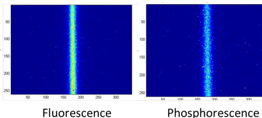
*Figure 2: Fluorescence and phosphorescence signals of argon-acetone mixture at atmospheric pressure*
