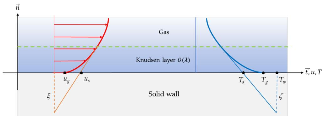
Figure 1 : Velocity slip and Temperature jump in the slip-flow regime.
