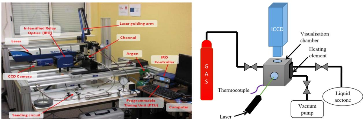
Figure 4: MT experimental setup developed at ICA for velocimetry (left) and thermometry (right)
