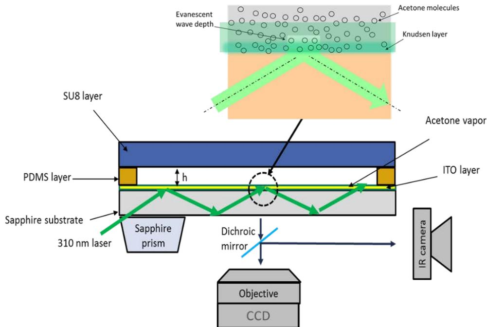
Figure 3: Principle of expected experimental setup
